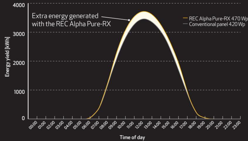
Calculations based on simulation results for full calendar year, based on an 12 kWp system in Palm Springs, CA, USA. Peak REC Alpha Pure-RX energy yield difference at midday: +6%, with an overall greater annual yield of 5.4w%. Performance may vary dependent on location.
